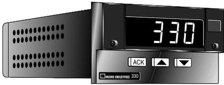
The 330 is a process monitor with universal input that is multi-functional and microprocessor based. The 330 can function as a panel meter and trip (alarm), or as a panel meter with two trips (alarms), analog transmitter and digital transmission with the addition of the RS 485 serial communications option.
